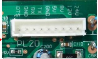
Power is supplied by the MOC to AOC via PL20. Do not disconnect to measure voltage
