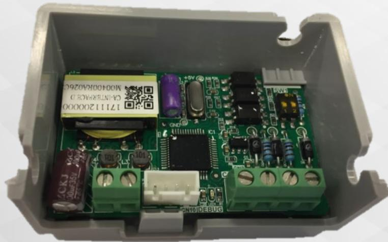
The Interface receives 24VAC signals for Cool, Heat, and Fan. This translates these commands to the system's communication protocol and sends the commands to indoor unit over the HA / HB communication bus.
