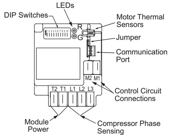
**Fig. 27 — Solid-State Motor Protection Module**
