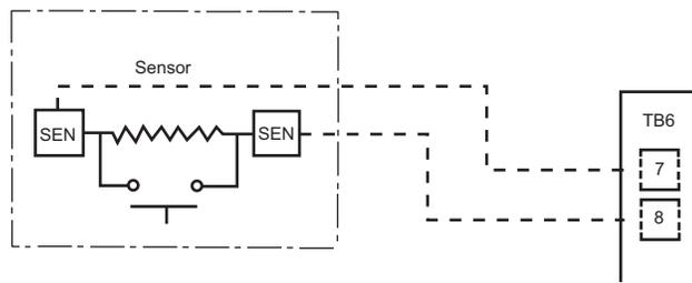
**Fig. 68 — Typical Space Temperature Sensor (33ZCT55SPT) Wiring**
