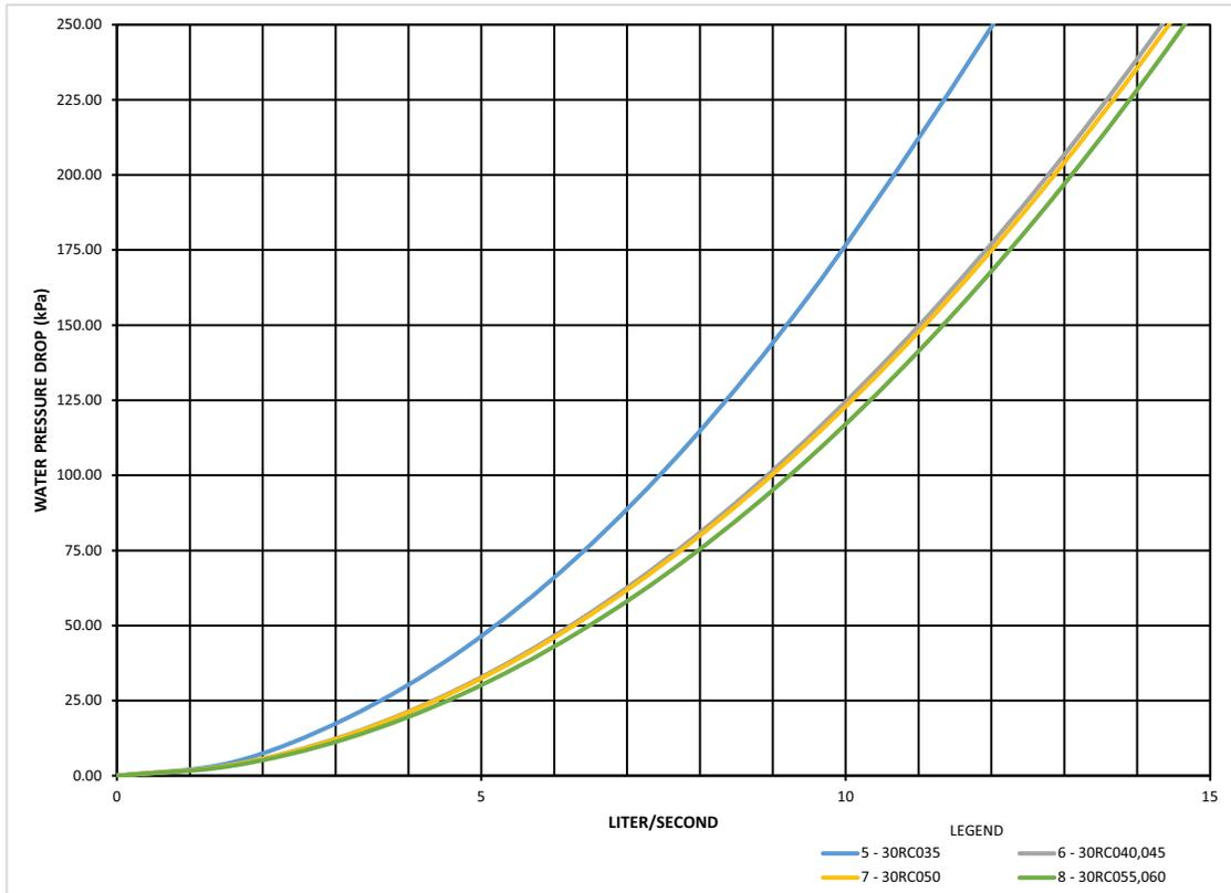
**Fig. 61 — 30RC 035-060 Single Pump Pressure Drop Curves (SI)**
