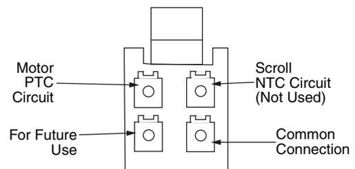
**Fig. 25 — CoreSense Communication Motor Thermistor Plug**
