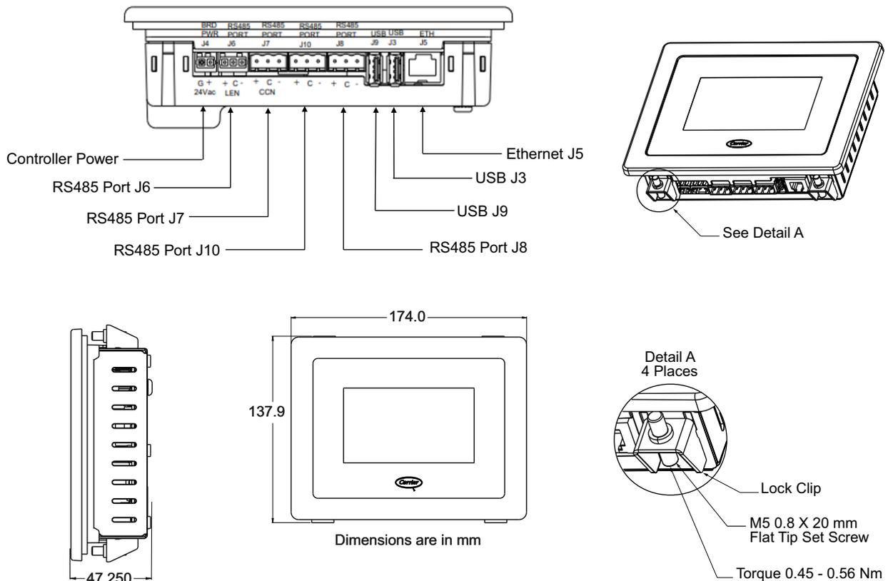
**Fig. 21 — Carrier Controller Display Interface and Connectors**
