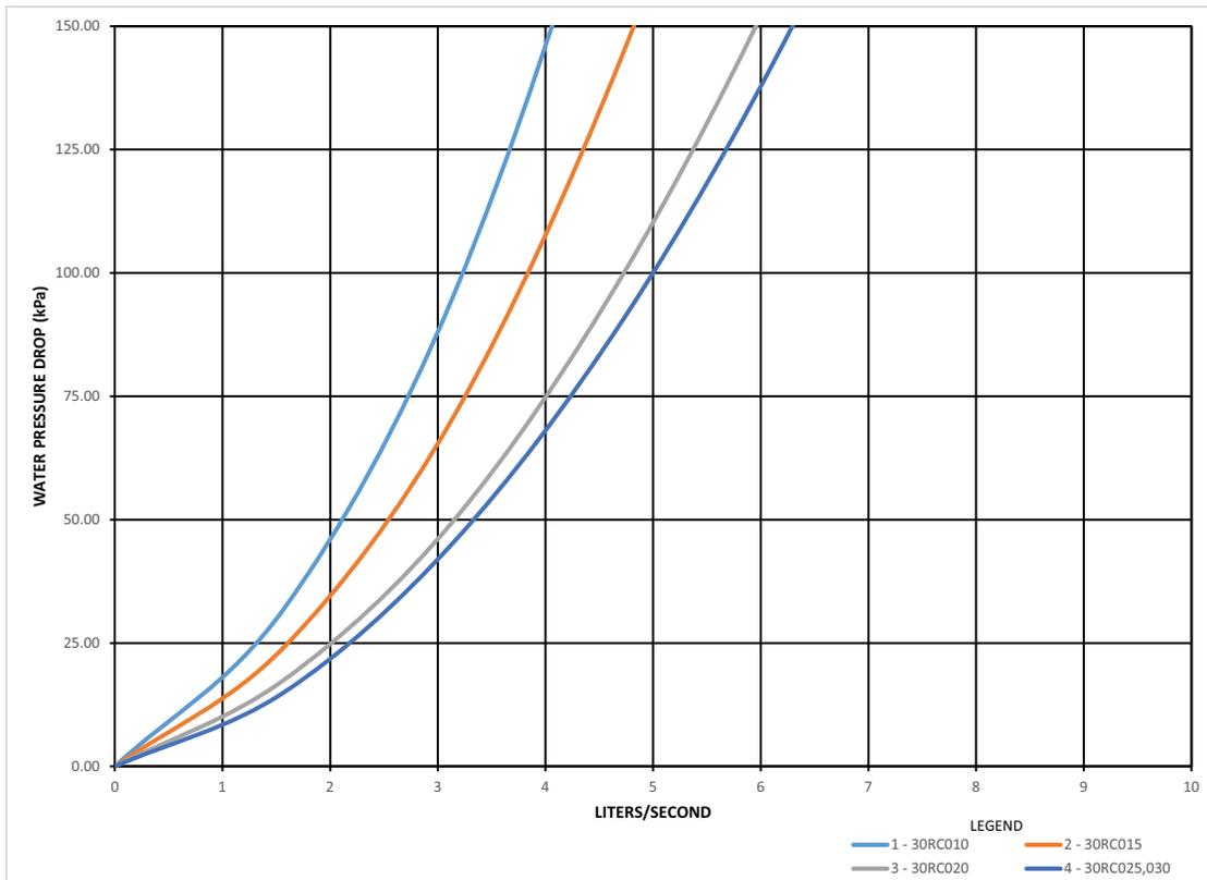
**Fig. 60 — 30RC 010-030 Single Pump Pressure Drop Curves (SI)**
