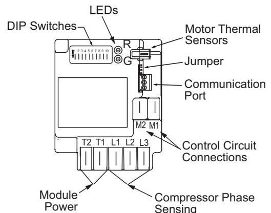
**Fig. 26 — CoreSense Communication Motor Protection Wiring**
