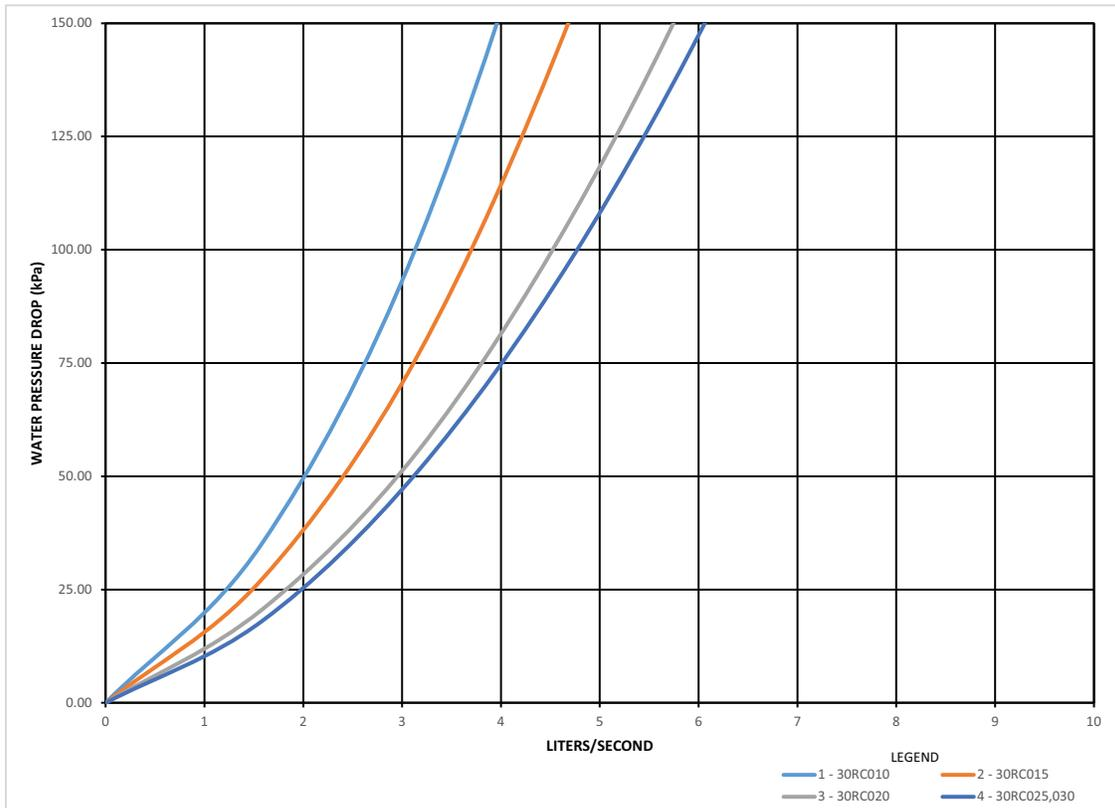
**Fig. 64 — 30RC 010-030 Dual Pump Pressure Drop Curves (SI)**
