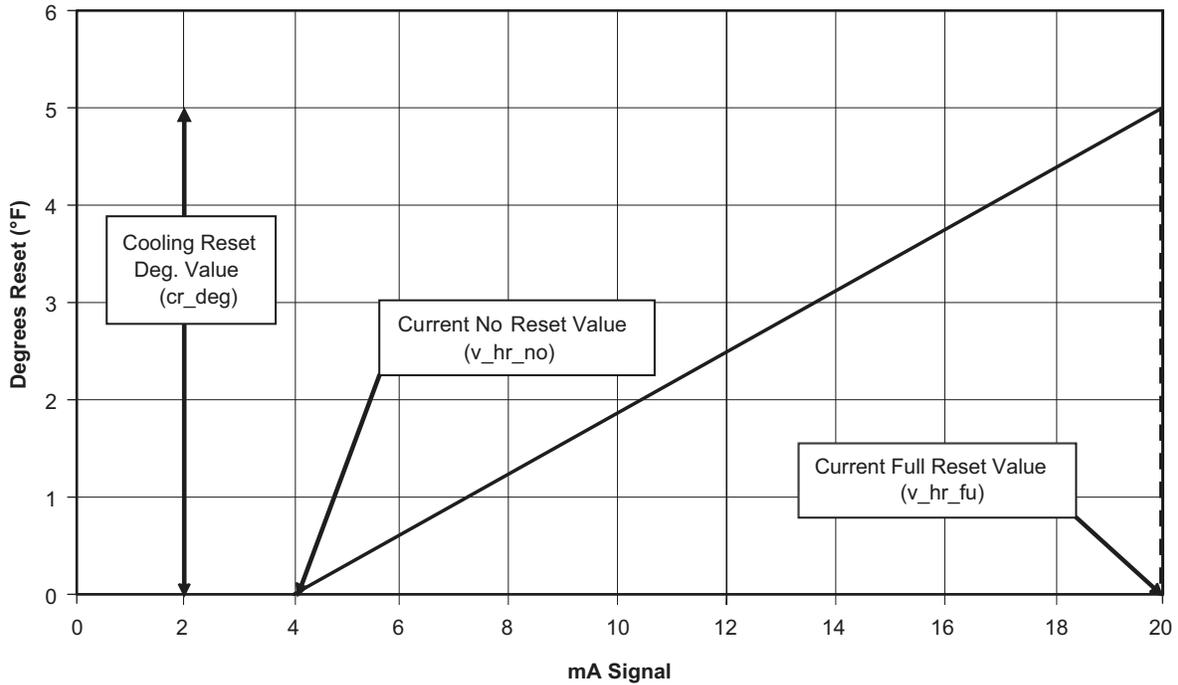
Fig. 44 — Example: 4 to 20 mA Temperature Reset
