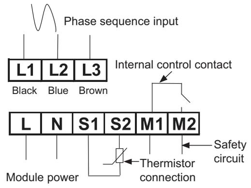
COPELAND COMPRESSORS MODELS WITH ELECTRICAL CODE “TW” OR “TE” (010-090) OR DANFOSS COMPRESSOR (100-150)
