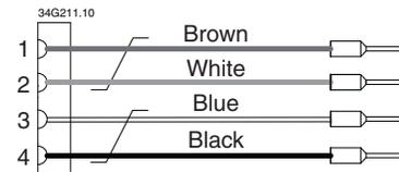
**Fig. 71 — EXV Pins and Wiring Connections**
