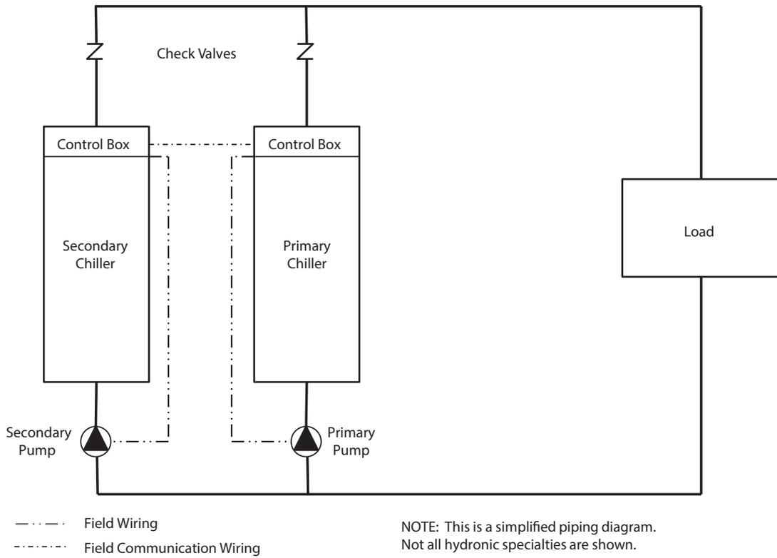
**Fig. 37 — Typical Parallel Primary/Secondary Chillers
