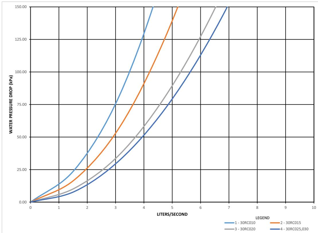
**Fig. 56 — 30RC 010-030 Unit Pressure Drop Curves (SI)**
