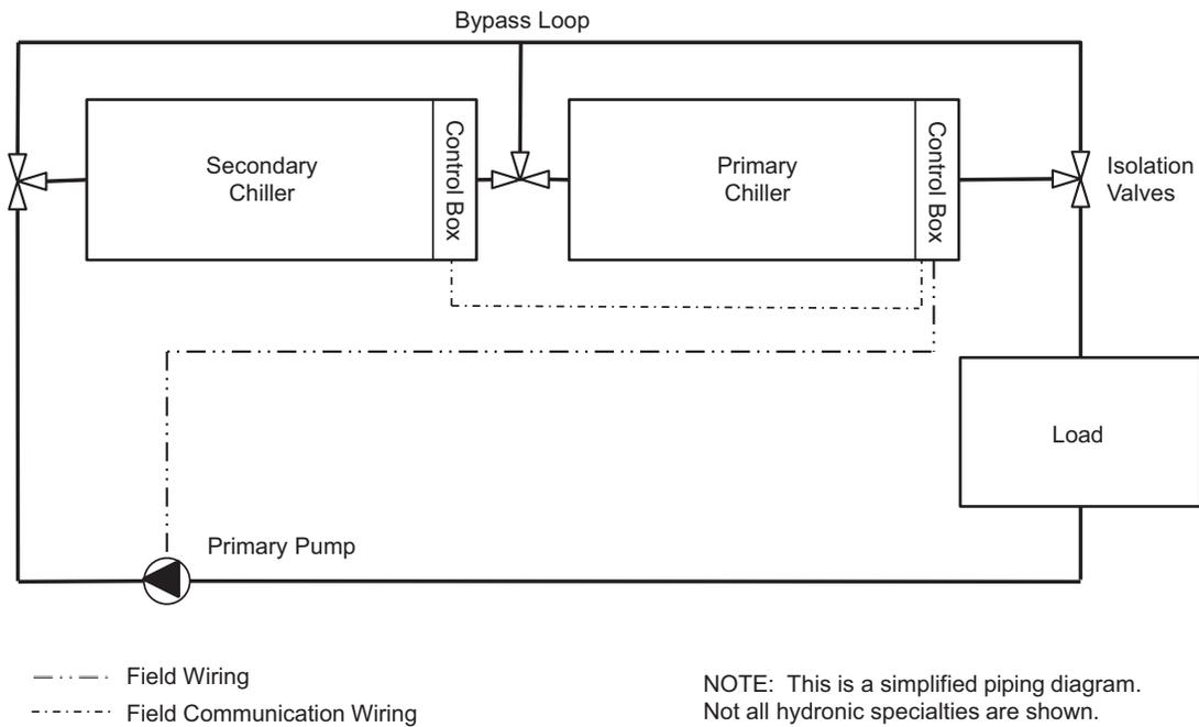
**Fig. 39 — Typical Series Primary/Secondary Chillers
