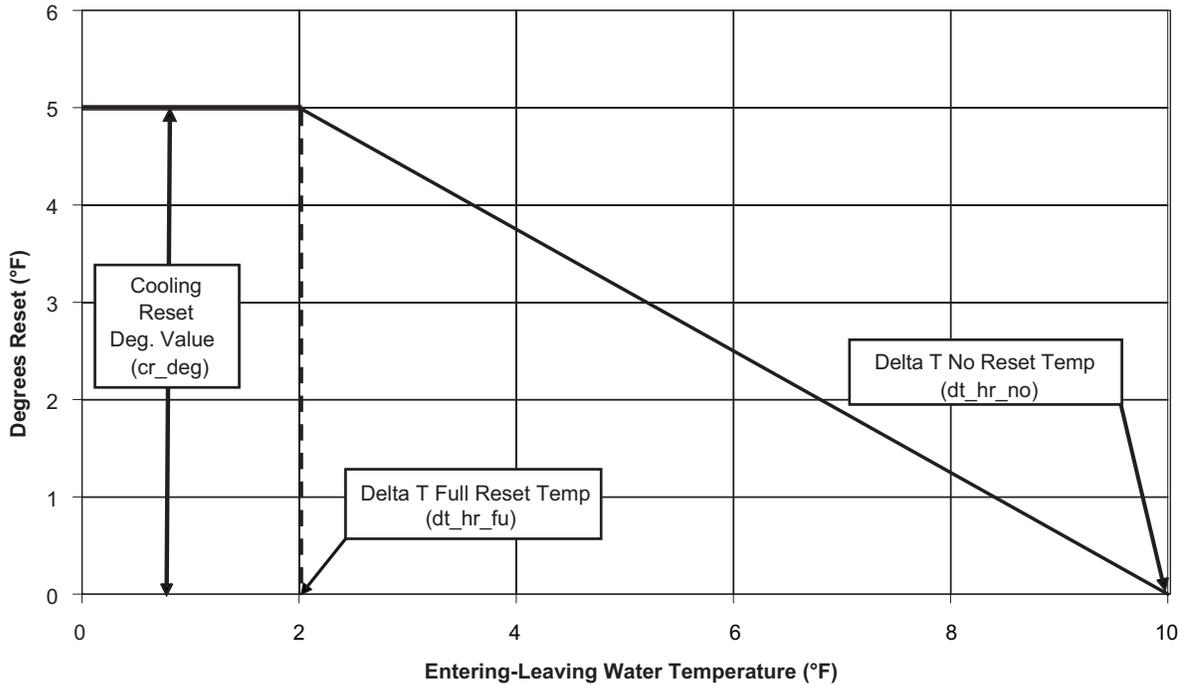
**Fig. 43 — Example: Return Water Reset**
