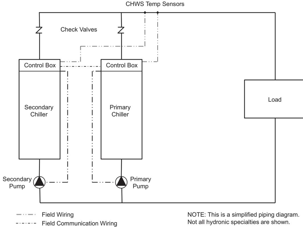
**Fig. 35 — Typical Parallel Primary/Secondary Chillers
