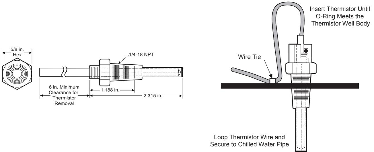
**Fig. 67 — Dual Chiller Accessory Kit Leaving Water Thermistor and Well (P/N 00EFN900044000A)**
