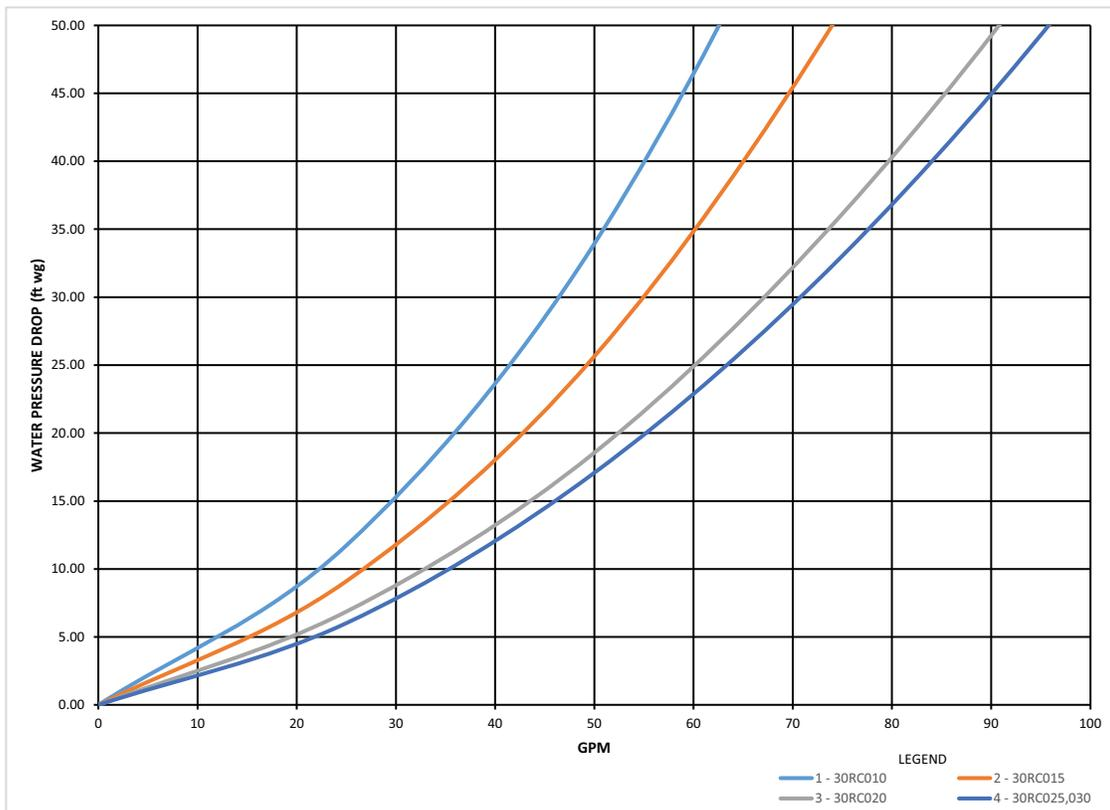
**Fig. 62 — 30RC 010-030 Dual Pump Pressure Drop Curves (English)**
