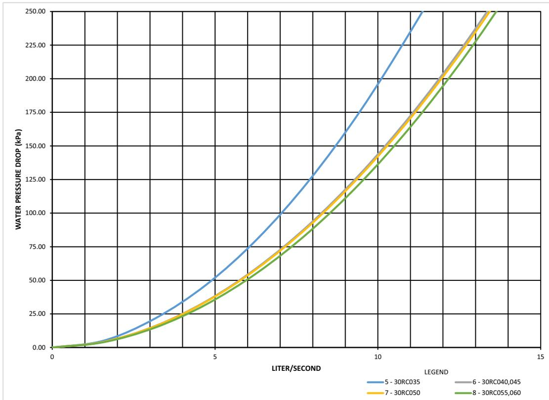
Fig. 65 — 30RC 035-060 Dual Pump Pressure Drop Curves (SI)
