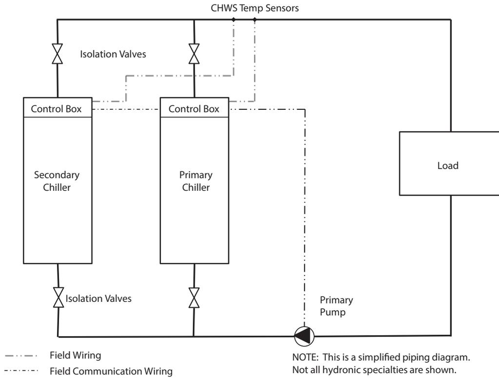
**Fig. 36 — Typical Parallel Primary/Secondary Chillers
