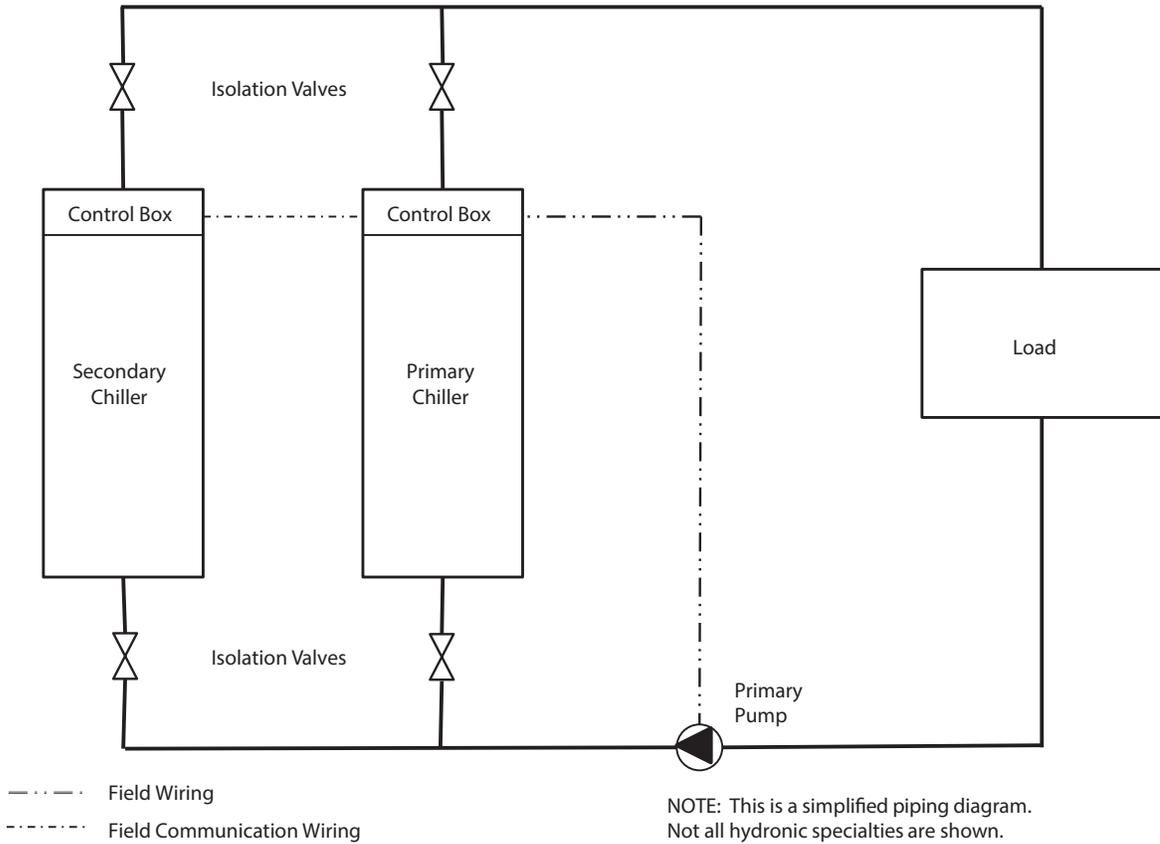
**Fig. 38 — Typical Parallel Primary/Secondary Chillers
