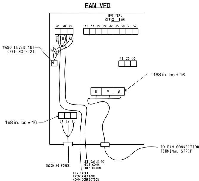
**Fig. 78 — Fan Drive Wiring**
