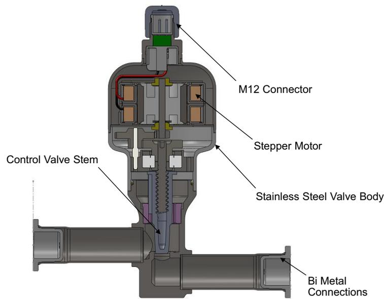
**Fig. 70 — Cutaway View of the Electronic Expansion Valve**
