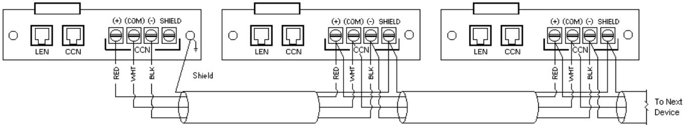
**Fig. 29 — Carrier Controller CCN Communication Wiring**
