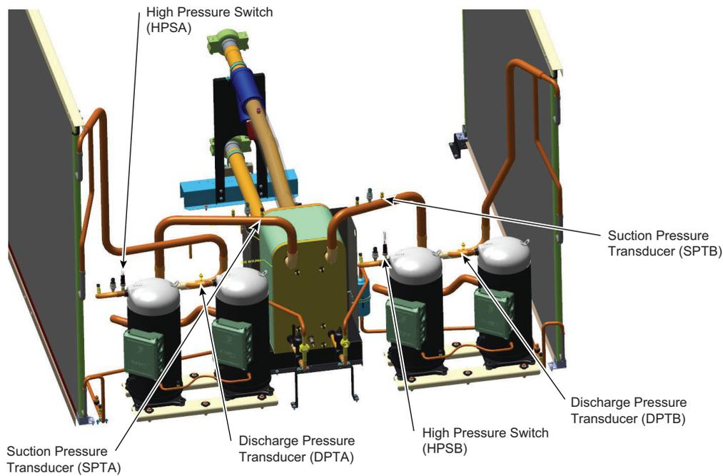
**Fig. 69 — Transducer and Switch Locations**
