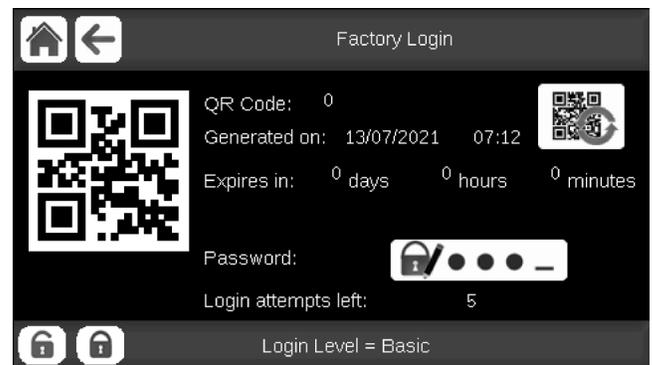
**Fig. 6 — Factory Login Level Screen**
