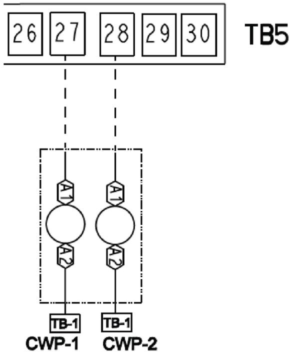
**Fig. 34 — Wiring for Evaporator Pump Control**
