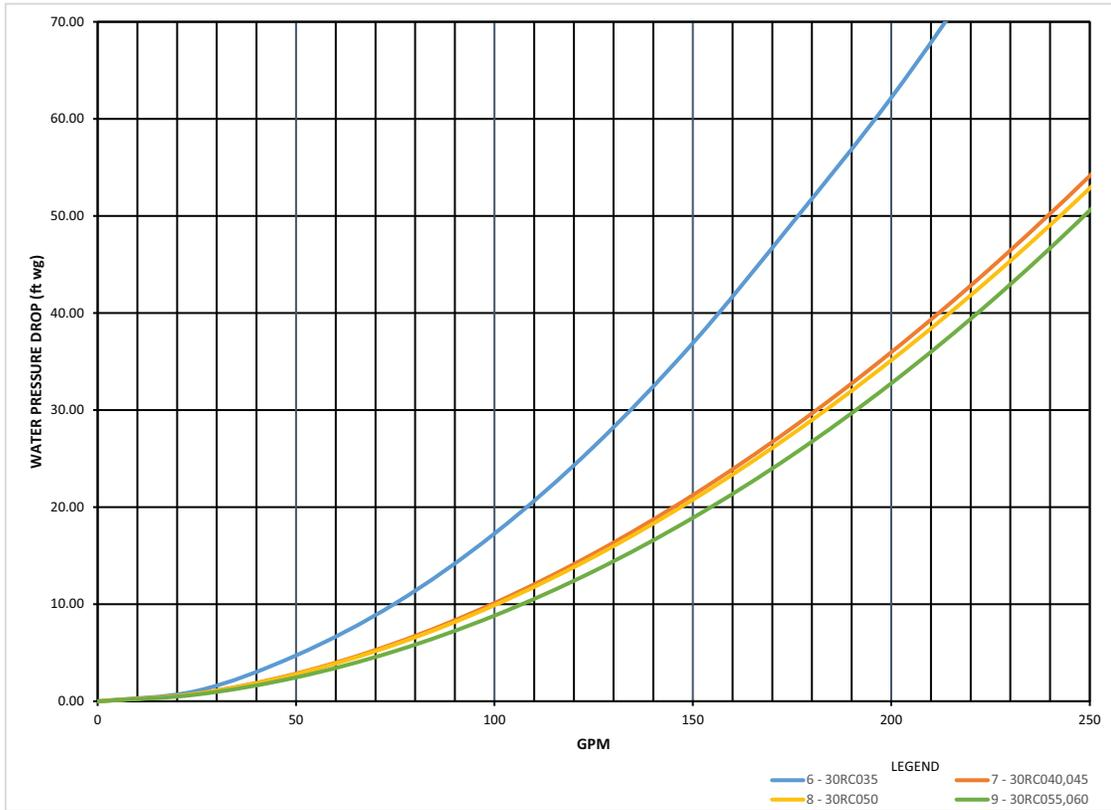
**Fig. 55 — 30RC 035-060 Unit Pressure Drop Curves (English)**
