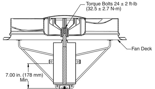
Fig. 75 — AeroAcoustic Fan (Black Bolt) Mounted Position
