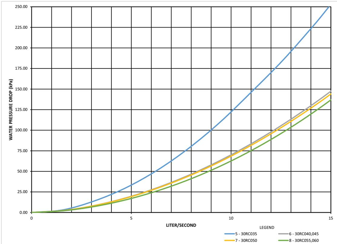
**Fig. 57 — 30RC 035-060 Unit Pressure Drop Curves (SI)**
