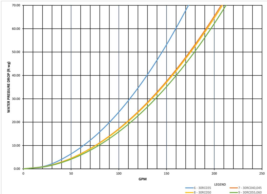
**Fig. 59 — 30RC 035-060 Single Pump Pressure Drop Curves (English)**
