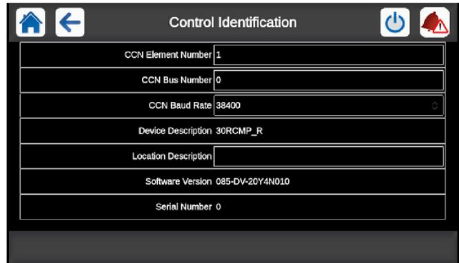
**Fig. 30 — CCN Control Identification Screen**
