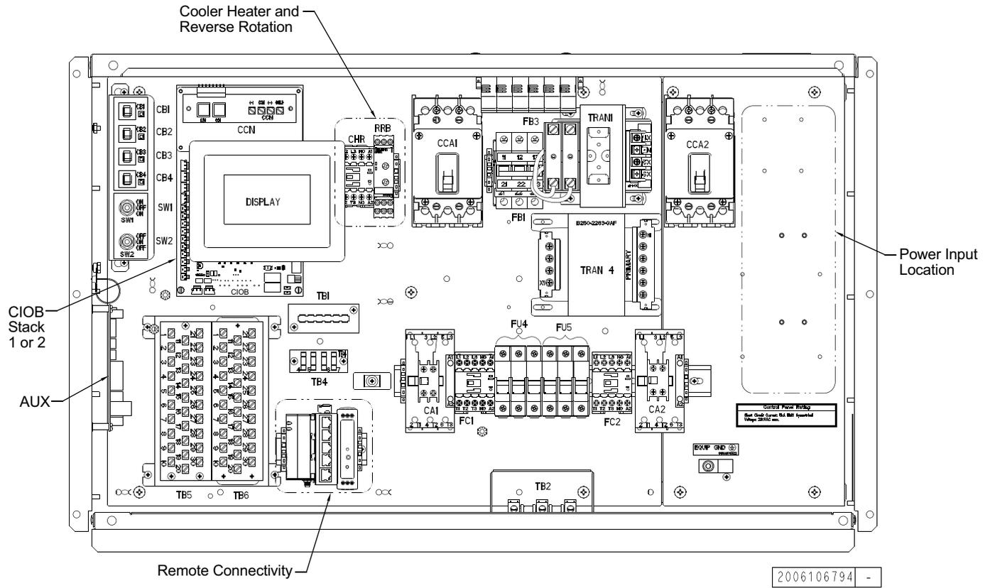
**Fig. 1 — Component Layout Drawing (30RC010-030 — Small Main)**
