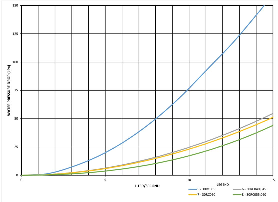
**Fig. 53 — 30RC 035-060 BPHE Pressure Drop Curves (SI)**
