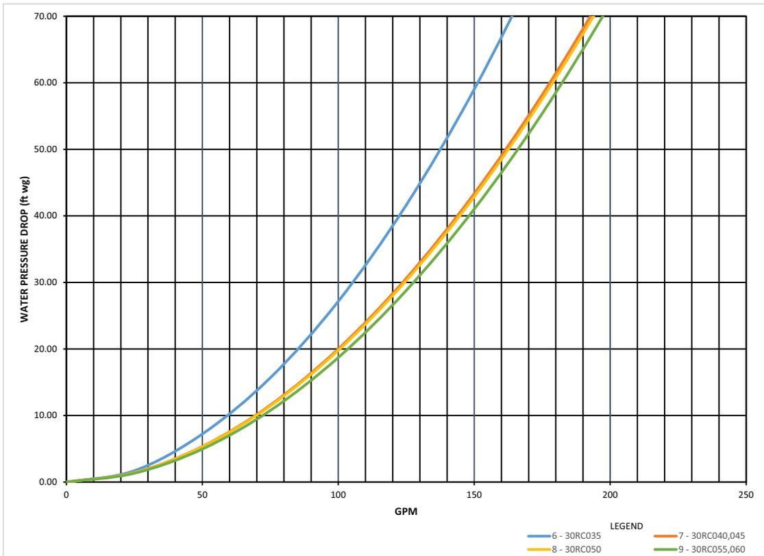
**Fig. 63 — 30RC 035-060 Dual Pump Pressure Drop Curves (English)**
