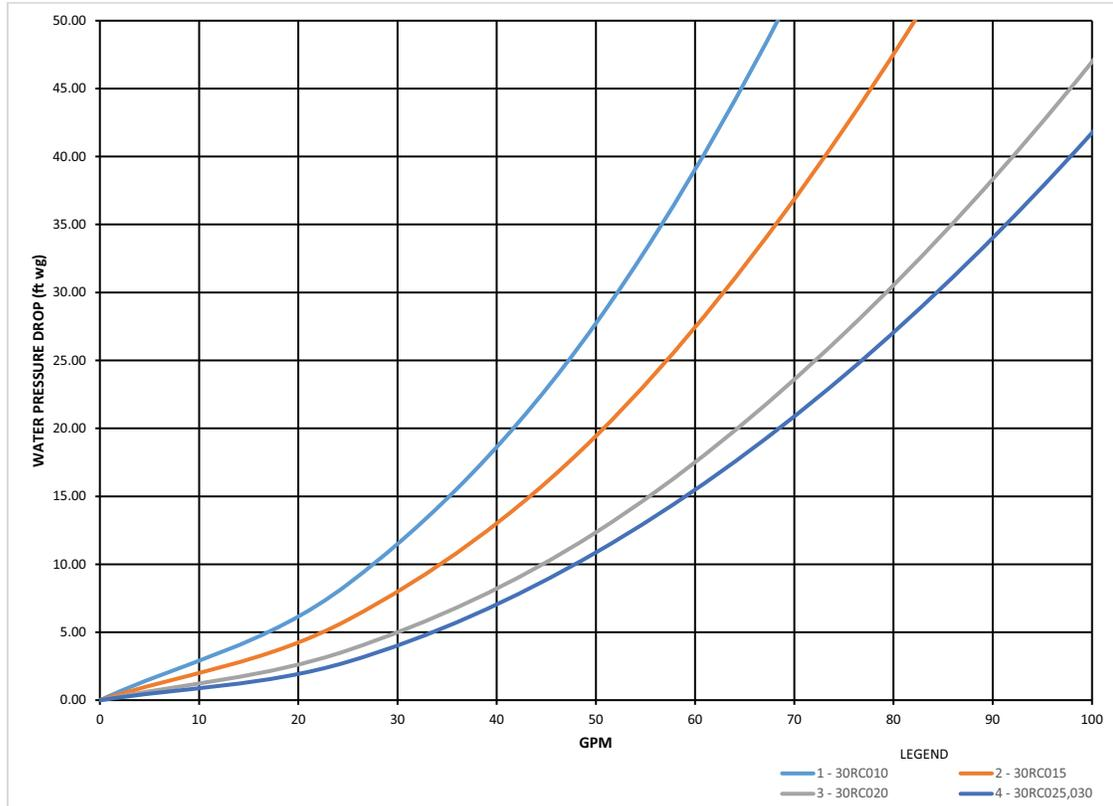
**Fig. 54 — 30RC 010-030 Unit Pressure Drop Curves (English)**
