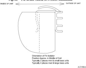
Fig. 34 – Fin Isolator Orientation
