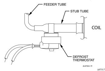
Fig. 9 - Defrost Thermostat Location
