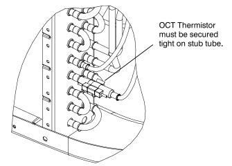
Fig. 47 - Outdoor Coil Thermistor (OCT) Attachment
