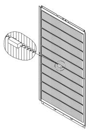
Fig. 3 – Louver Spacer Location
