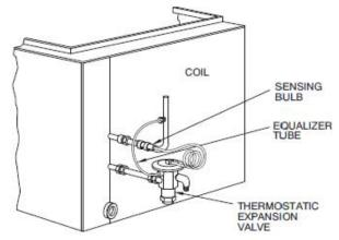
Fig. 29 - Typical TXV Installation
