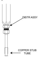
Fig. 35 – Copper Stub Tube Connection
