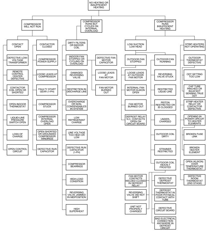
Fig. 51 – Heat Pump Troubleshooting - Heating Cycle
