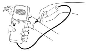
Fig. 30 - Electronic Leak Detection
