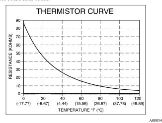
Fig. 43 – Resistance Values Versus Temperature
