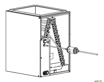
Fig. 25 – Liquid Line Filter Drier - AC
