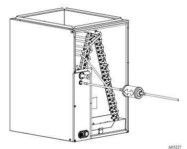
Fig. 26 - Liquid Line Filter Drier - HP
