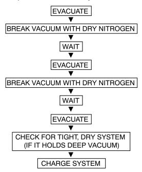
Fig. 37 – Triple Evacuation Method
