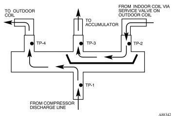
Fig. 23 – Reversing Valve (Cooling Mode or Defrost Mode, Solenoid Energized)
