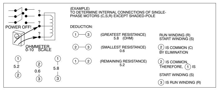
Fig. 19 – Identifying Compressor Terminals
