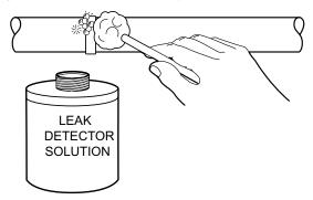
Fig. 31 - Bubble Leak Detection
