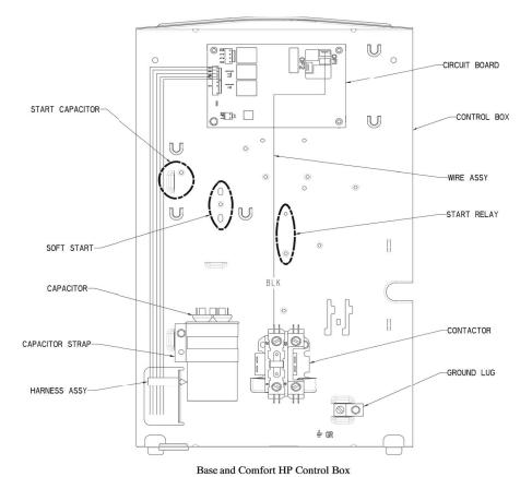
Fig. 4 – Base and Comfort Series Control Box Identification
