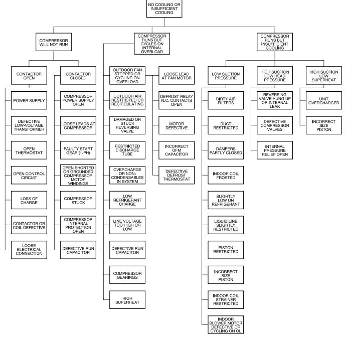
Fig. 52 - Heat Pump Troubleshooting - Cooling Cycle
