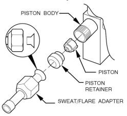
Fig. 22 – AccuRaterr Components (used in R-22 Heat Pumps)
