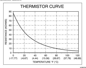
Fig. 42 – Resistance vs. Temperature Chart
