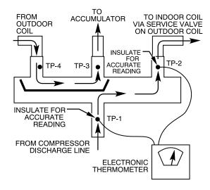
Fig. 24 – Reversing Valve (Heating Mode, Solenoid De-Energized)
