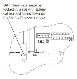
Fig. 46 – Outdoor Air Thermistor (OAT) Attachment
