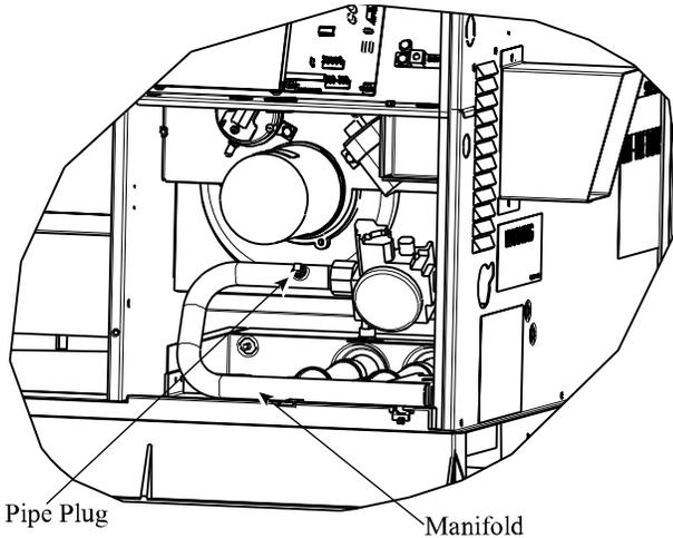
Fig. 39 – Burner Assembly
