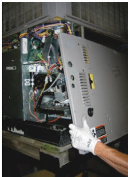
**Fig. 37 – Replacing Right Side Panel** A210081
