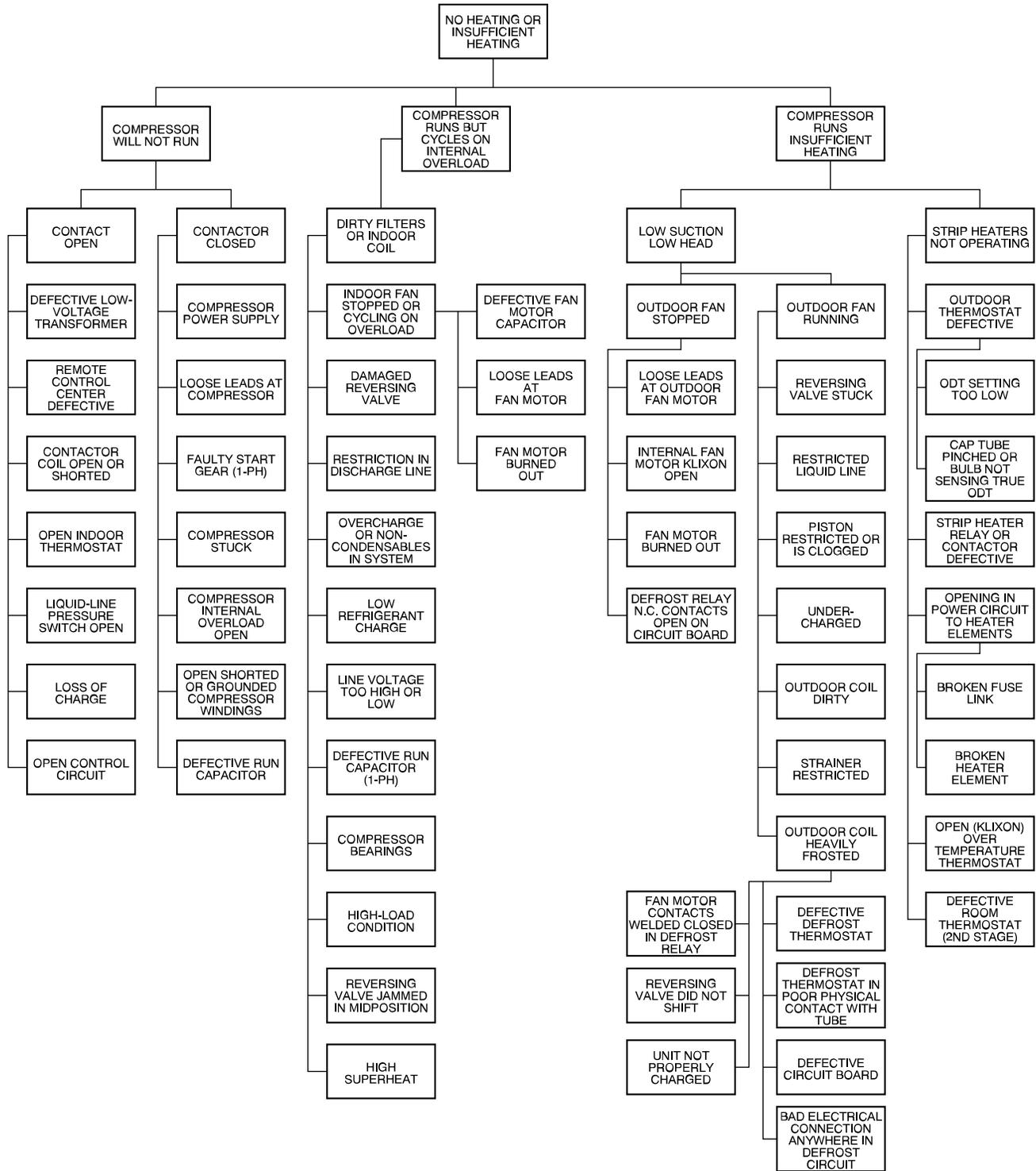
Fig. 48 – Heat Pump Troubleshooting - Heating Cycle
