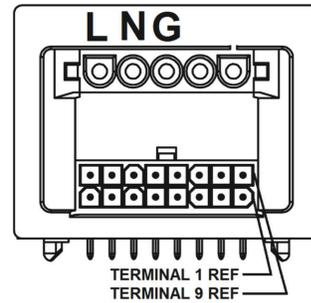
Fig. 26 – EON™ Module Plug (Advanced Dehumidification Models)
