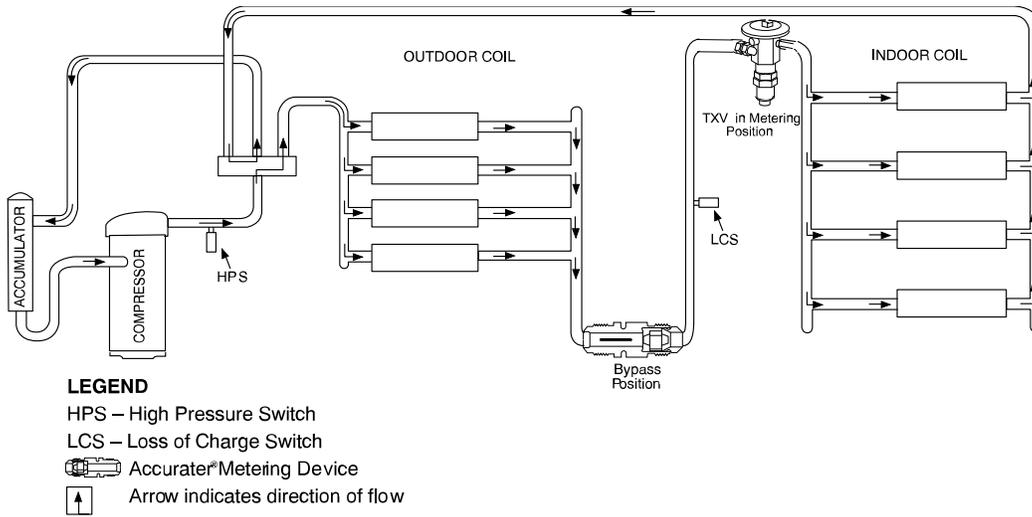
Fig. 45 – Typical Heat Pump Operation, Cooling Mode
