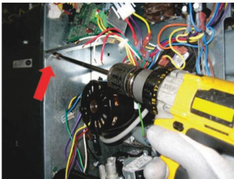
**Fig. 34 – Removing Screw Under Control Board Panel** A210078
