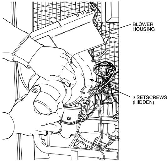
Fig. 43 – Removal of Motor and Blower Wheel
