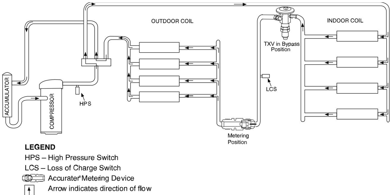
Fig. 46 – Typical Heat Pump Operation, Heating Mode
