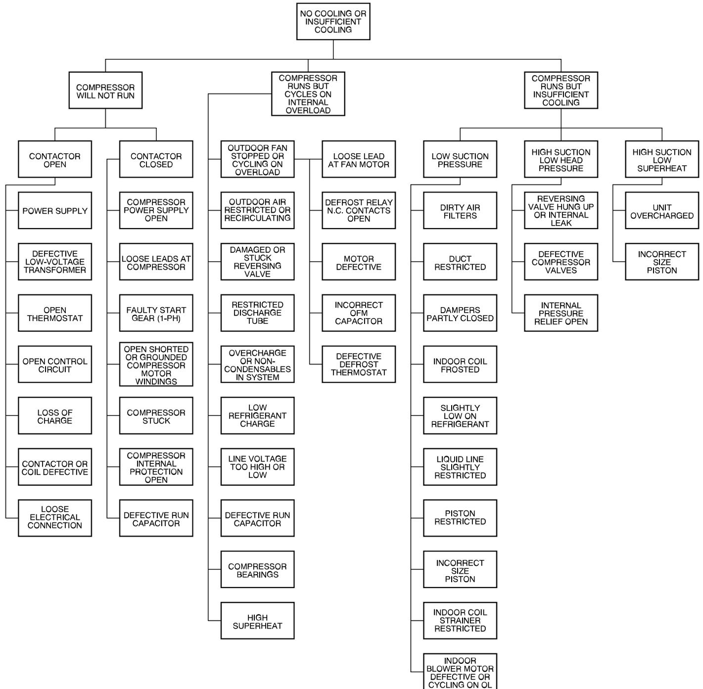
Fig. 49 – Heat Pump Troubleshooting - Cooling Cycle
