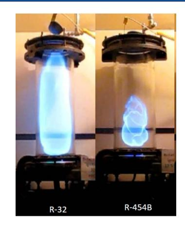
R32 reached top of cylinder in 0.233 seconds(Note stopper release at top)
