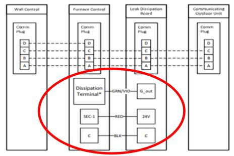
**NOTE**: Dissipation terminal is only used on Carrier communicating furnaces manufactured Q4 2023 and later. Use a 3/16" spade connector on the GRN/VIO wire to connect to the dissipation terminal on communicating furnaces. Attach wire nut to all unused wires from the power harness.
