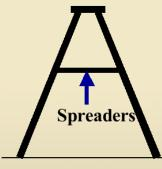
Check For: ⇒Wear ⇒Cracks ⇒Damaged Parts ⇒Missing Parts ⇒Loose Component
